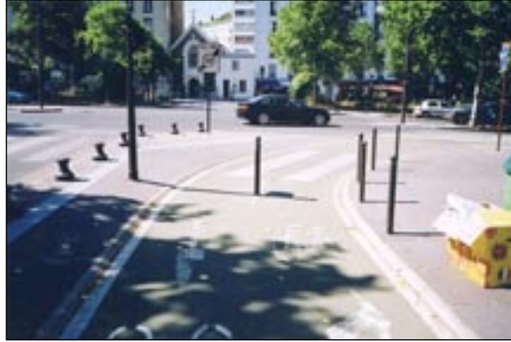
Two-way bike traffic with well-placed bollard to stop large vehicles
