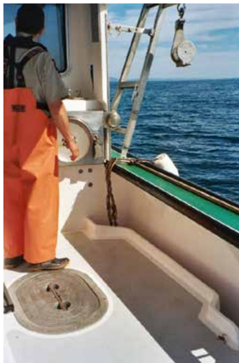
Rope locker built-in to the Maine Marine Patrol vessel Guardian III to reduce the risk of entanglement in trap rope. Photo by Ann Backus, Rockland, Maine, August 2004.
