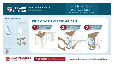
Reduce your indoor exposure to COVID-19. Learn how to make a portable do-it-yourself prism air cleaner with a circular fan to remove contaminants such as viruses from the air.
