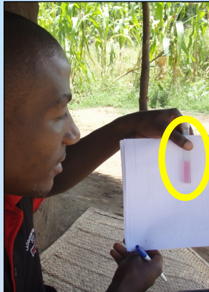
Positive test for chlorine in stored water
